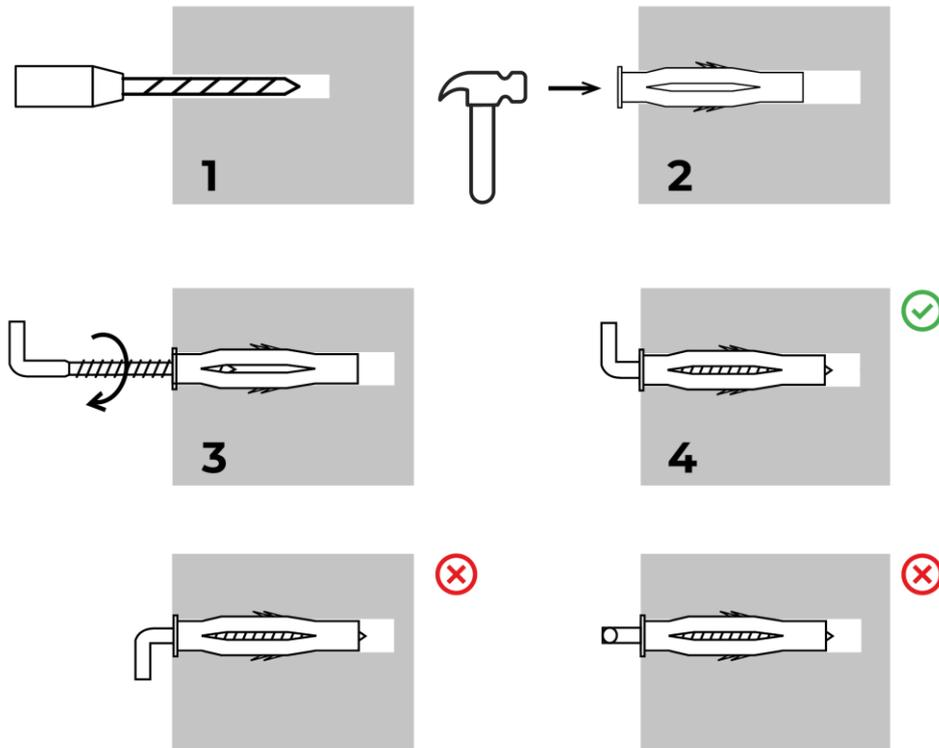
The process of screwing in the hooks
