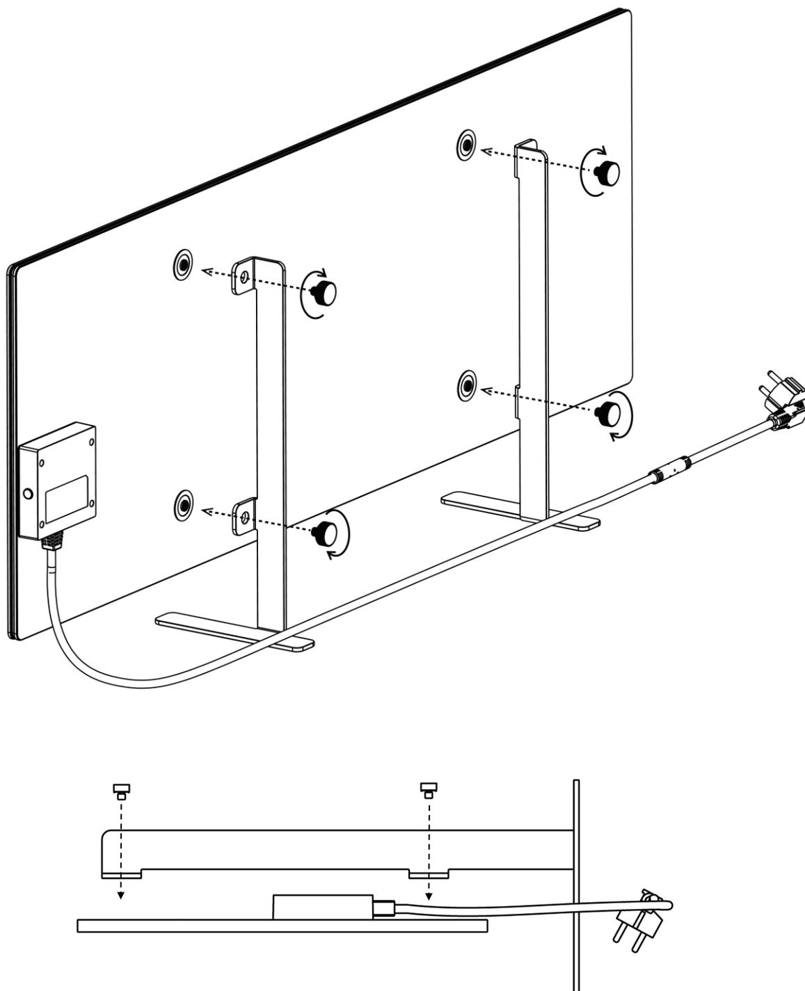
Figure 6 – Mounting on legs (on the floor)
