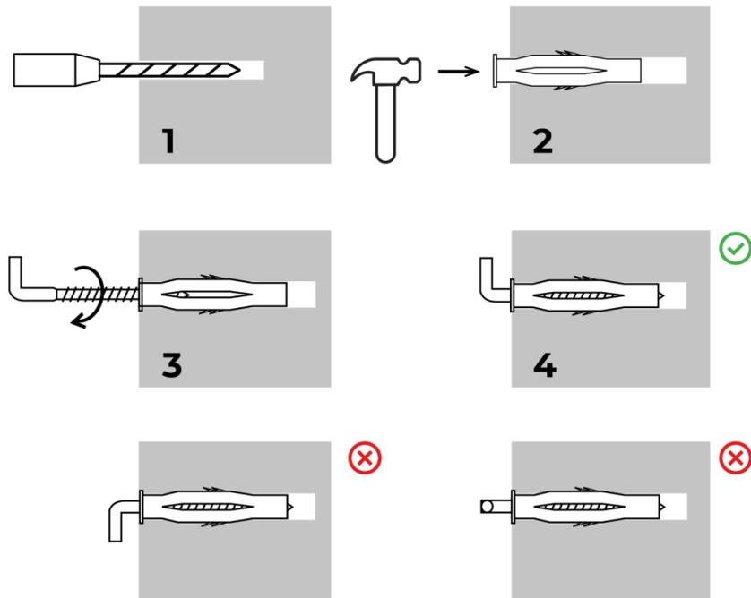
The process of screwing in the hooks
