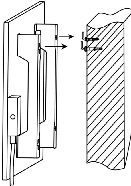
5. Check that the device is securely fixed.
